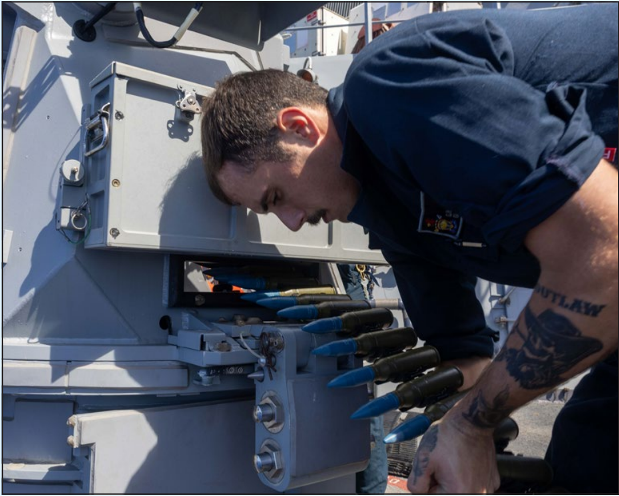
U.S. Navy photo by Mass Communication Specialist 2nd Class Ange Olivier Clement Seaman Gabriel Blankenship of Fishers uploads ammunition into a Mark .38 25 mm machine gun system during routine operations aboard the Arleigh Burke-class guided-missile destroyer USS Milius (DDG 69), in the Pacific Ocean on Nov. 14. Milius is forward-deployed and assigned to Destroyer Squadron (DESRON) 15, the Navy's largest DESRON and the U.S. 7th Fleet's principal surface force.
