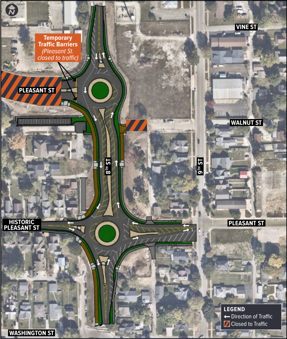
8th Street roundabouts will be open to traffic temporarily as single lane roundabouts. The final asphalt surface and striping will be completed prior to Phase 1 completion in 2024. Graphic provided by American Structurepoint
