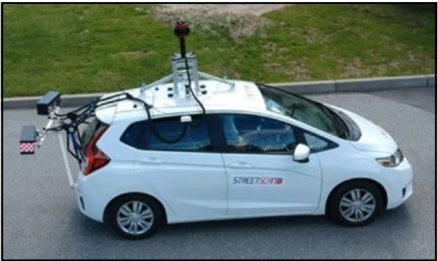
Photo provided This StreetScan car will use sensors to detect and assess the conditions of Carmel's roads.
