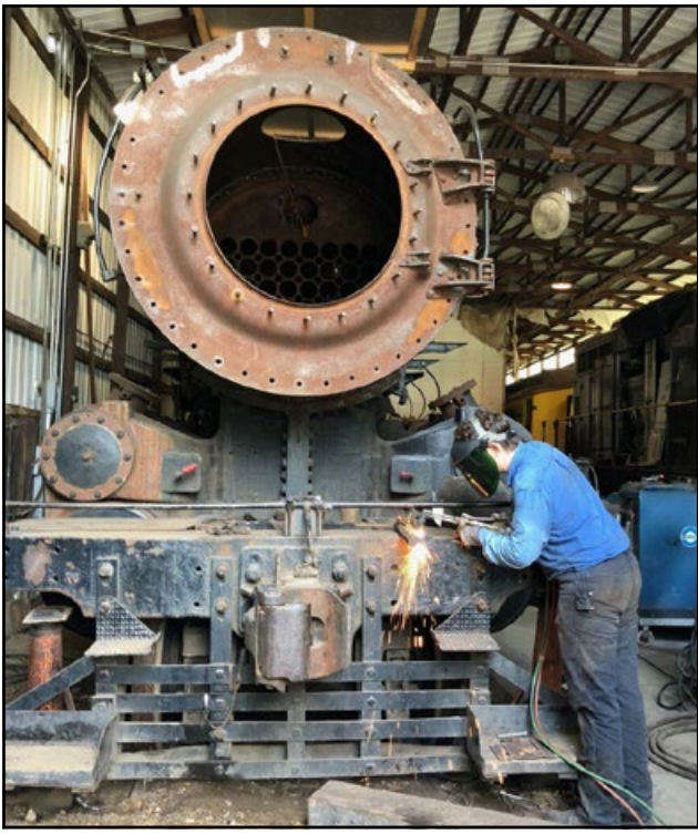
(Left) Jason Sobczynski of Kentucky Steam Heritage Corp. creates makeshift bracing to prepare the 587 steam locomotive for transport and removal from Forest Park. (Right) Members of the Indiana Transportation Museum work on the emergency rescue of a steam locomotive from the ITM back shops.
